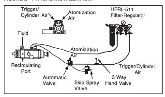
Attach the trigger/cylinder air hose and the atomization air hose to the connections as indicated by the markings on the gun body. The air supply should be filtered and regulated. Attach the material hose to the fluid inlet on the gun body. Fluid can be recirculated by installing a fluid fitting (AGX-415) (order separately) at the recirculating port. See **Caution** below.
